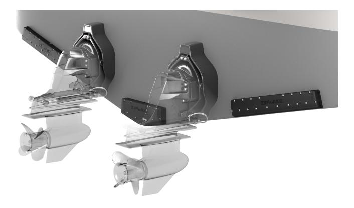
Centerline mounted interceptors can be included in new installations, or retro-fitted to already installed systems.
